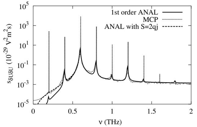
**Figure 7.** First-order iteration for  $S_{U_d U_d}(\omega)$  (solid line) in comparison with the MCP results and first-order iteration with the improved shot-noise level (dotted and dashed lines, respectively).  $R = 10^{-8} \text{ } \Omega \text{ m}^2$ ,  $U_0 = 0.6 \text{ V}$ ,  $U_1 = 0.2 \text{ V}$ ,  $\nu_0 = 200 \text{ GHz}$  and  $T = 500 \text{ ps}$ .
