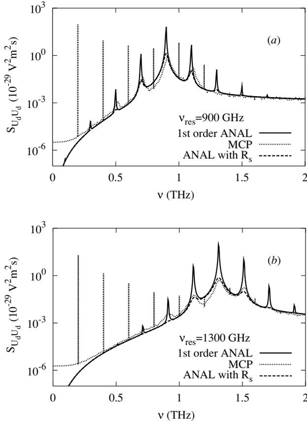
**Figure 8.** Spectral densities of the total voltage drop on the load resistor  $R$  calculated by the MCP technique (dotted curves) and by the analytical approach in the first-order approximation without and with the spreading resistance (solid and dashed lines, respectively) for two values of  $\nu_{\text{res}}$ : (a) 900 and (b) 1300 GHz.  $U_0 = 0.6$  V,  $U_1 = 0.2$  V,  $\nu_0 = 200$  GHz,  $R = 10^{-8} \Omega \text{ m}^2$  and  $T = 2$  ns.
