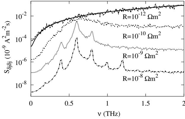
**Figure 2.** Spectral density of current fluctuations through load resistance  $R = 10^{-12}, 10^{-10}, 10^{-9}$  and  $10^{-8} \Omega \text{ m}^2$  calculated at  $U_0 = 0.6 \text{ V}, U_1 = 0.2 \text{ V}$  and  $\nu_0 = 200 \text{ GHz}$  when the parallel circuit exhibits a resonance at the third harmonic.
