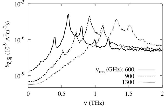
**Figure 3.** Spectral density of current fluctuations through the load resistance  $R = 10^{-8} \Omega \text{ m}^2$  calculated at  $U_0 = 0.6 \text{ V}, U_1 = 0.2 \text{ V}$  and  $\nu_0 = 200 \text{ GHz}$ , and different  $\nu_{\text{res}} = 600, 900$  and  $1300 \text{ GHz}$  to which the parallel resonant circuit is tuned.
