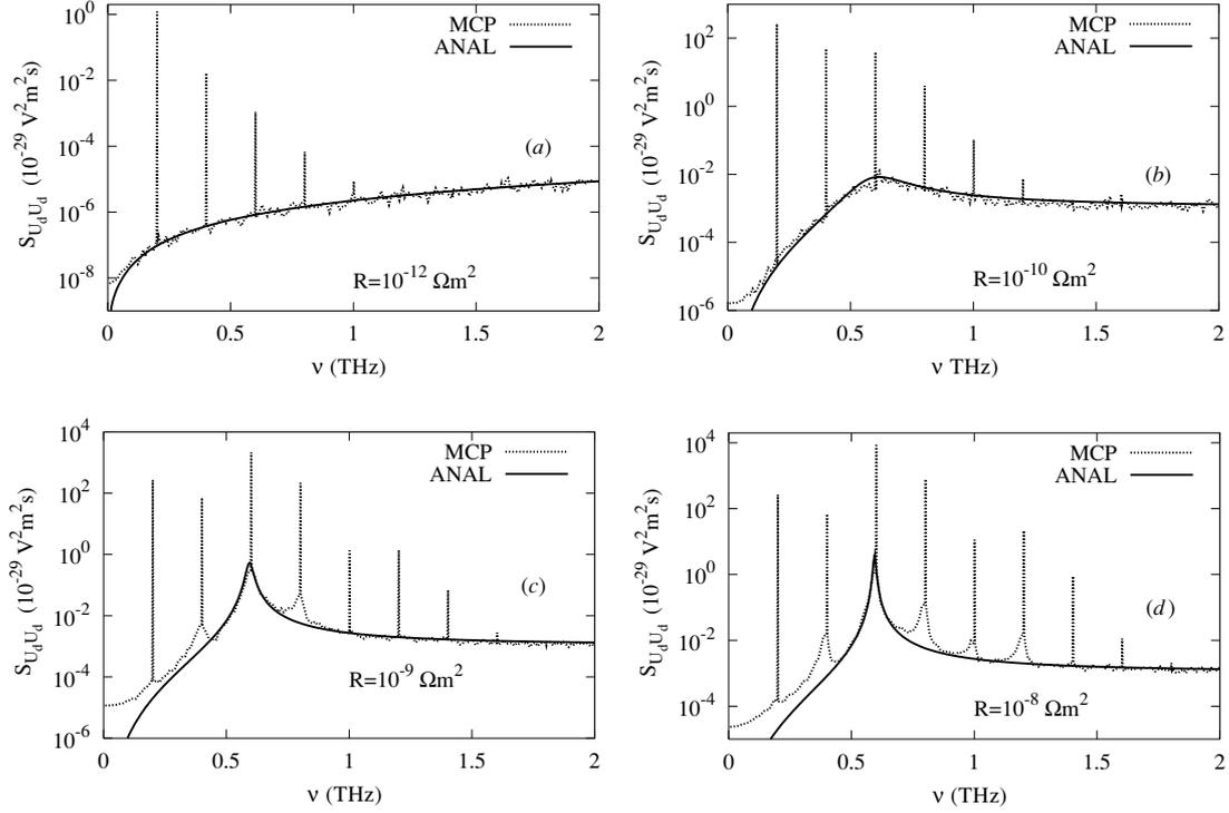
**Figure 5.** Spectral densities of the total voltage drop on the load resistor  $R$  calculated by the MCP technique (dotted curves) and by the analytical approach in the zero-order approximation (solid lines) for different values of  $R$ : (a)  $R = 10^{-12} \Omega\text{m}^2$ , (b)  $10^{-10}$ , (c)  $10^{-9}$  and (d)  $10^{-8} \Omega\text{m}^2$ .  $U_0 = 0.6\text{ V}$ ,  $U_1 = 0.2\text{ V}$  and  $\nu_0 = 200\text{ GHz}$ .
