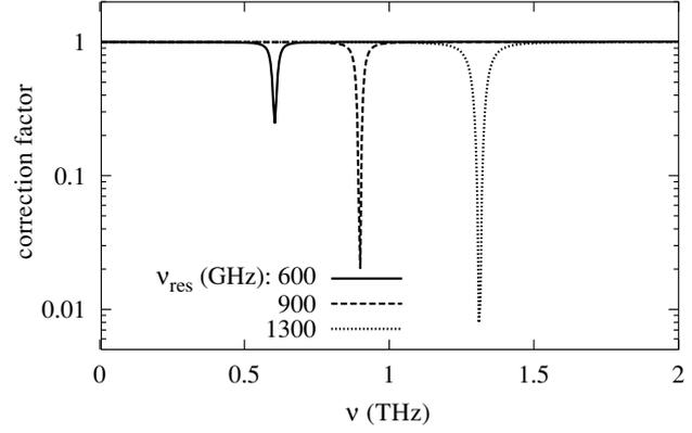
**Figure 9.** Frequency dependence of the correction factor caused by the spreading resistance  $R_s = 10^{-12} \Omega \text{ m}^2$  for the zero-order approximation at different values of  $\nu_{\text{res}}$ .  $U_0 = 0.6$  V,  $U_1 = 0.2$  V,  $\nu_0 = 200$  GHz and  $R = 10^{-8} \Omega \text{ m}^2$ .
