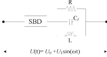
**Figure 1.** Scheme of the series connection of the SBD with a parallel resonant circuit.
