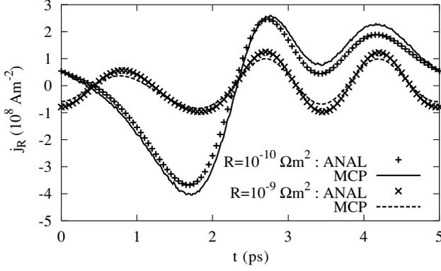
**Figure 4.** The regular part of the current flowing through the load resistance as a function of the time corresponding to one period of the applied voltage. Calculations are performed with  $R = 10^{-10}$  and  $10^{-9} \Omega \text{ m}^2$  at  $U_0 = 0.6 \text{ V}$ ,  $U_1 = 0.2 \text{ V}$  and  $\nu_0 = 200 \text{ GHz}$ . Lines refer to MCP and symbols to analytically based approaches.
