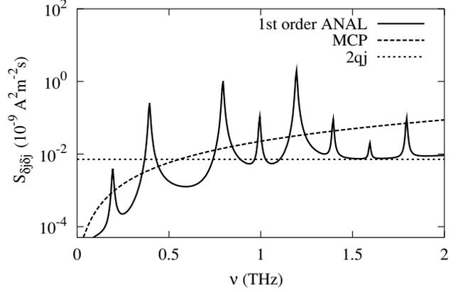
**Figure 6.** First-order iteration for the varactor component  $S_{jj}^v(\omega)$  (solid line) in comparison with the unperturbed spectral density of current fluctuations  $S_{jj}^d(\omega)$  (dashed line) and the shot-noise level under circuit operation (dotted line).  $U_0 = 0.6 \text{ V}$ ,  $U_1 = 0.2 \text{ V}$ ,  $\nu_0 = 200 \text{ GHz}$  and  $R = 10^{-8} \text{ } \Omega \text{ m}^2$ .
