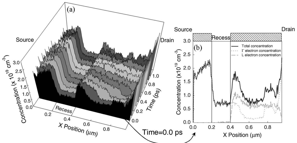
FIG. 5. (a) Profile of the carrier concentration in the channel of the heterostructure at different time moments within one period of the oscillation for a bias  $V_{DS}=1.0$  V. (b) Profile of the  $\Gamma$  valley (dotted line),  $L$  valley (dashed line), and total carrier concentration (solid line) in the channel at a time of 0.0 ps.
