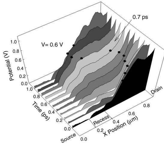
FIG. 6. Profile of the potential in the channel of the heterostructure at different time moments within one period of the oscillation for a bias  $V_{DS} = 1.0$  V. The point corresponding to  $V_{th} = 0.6$  V is marked in the different curves.
