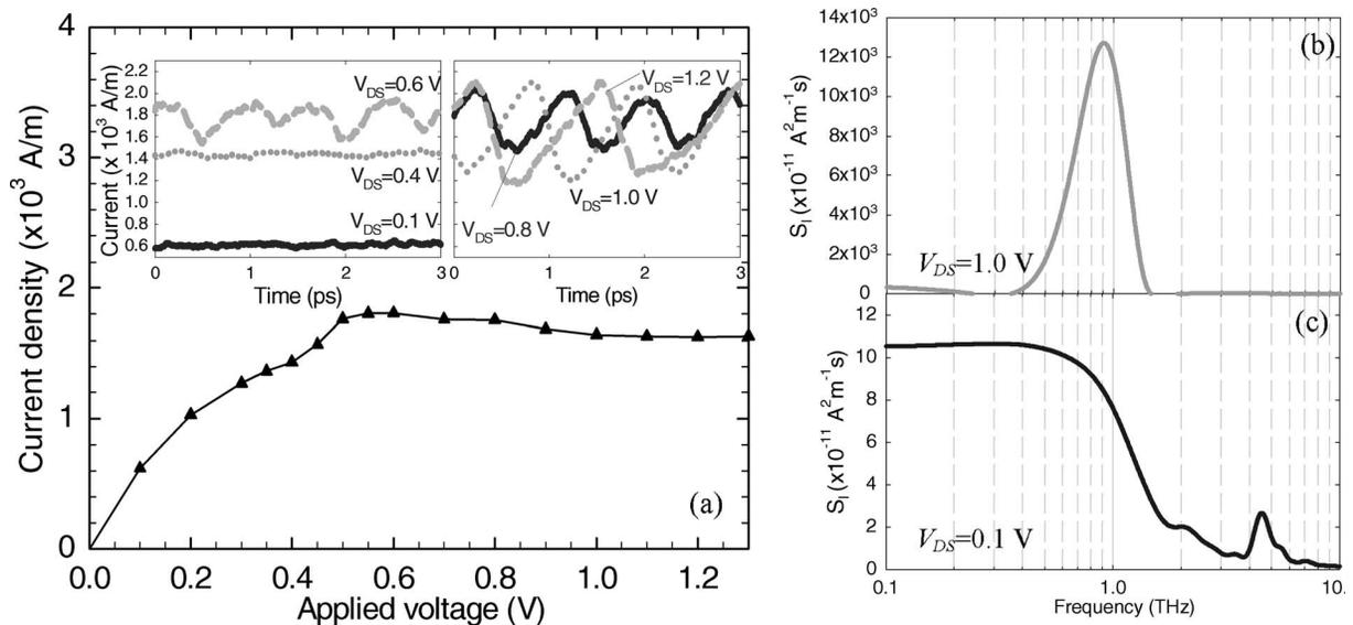
FIG. 2. (a) Static  $I$ - $V$  characteristic of the slot diode. The insets show the time-varying current for different applied voltages:  $V_{DS} \leq 0.6 \text{ V}$  (left inset) and  $V_{DS} > 0.6 \text{ V}$  (right inset). [(b) and (c)] Spectral density of current fluctuations for  $V_{DS} = 1.0 \text{ V}$  and  $V_{DS} = 0.1 \text{ V}$ , respectively.
