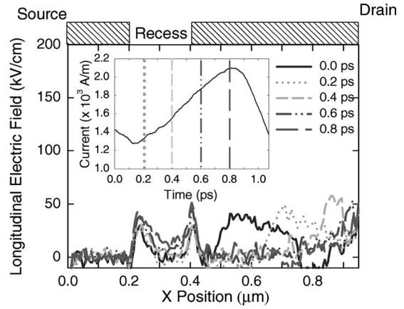
FIG. 4. Profile of the longitudinal electric field in the channel of the heterostructure at different time moments within one period of the oscillation for a bias  $V_{DS}=1.0$  V. The insets show the time-varying current during one period of the oscillation.
