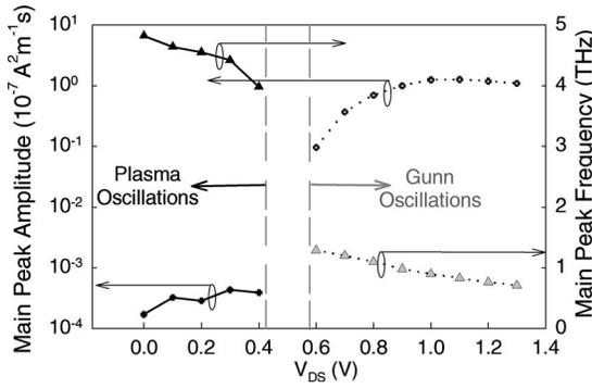
FIG. 3. Amplitude (crosses, left axes) and frequency (triangles, right axes) of the main peak in the spectral density of current fluctuations as a function of  $V_{DS}$ . The dotted lines indicate the  $V_{DS}$  regime where the Gunn oscillations take place.
