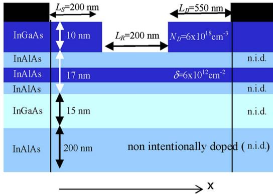
FIG. 1. (Color online) Geometry of the simulated InAlAs/InGaAs slot diode (note that the  $X$  axis is used in Figs. 4–6).
