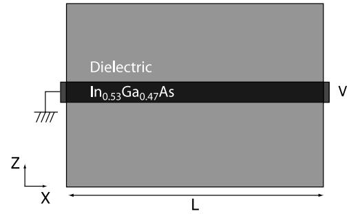
Figure 1. Schematic diagram of the device (not to scale) studied within the Monte Carlo simulation. The free charge is present only in the bar of length L along the x direction and thickness W along the z direction. The terminal at the left-hand side is the source contact kept at a voltage V = 0 the terminal at the right-hand side is the drain contact kept at a potential V . Carriers are reflected at the boundaries between the bar and the dielectric.
